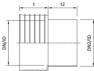
Table 10. Dimensions of Pecor Quattro/smooth-wall (e.g. PVC) pipe adapters
