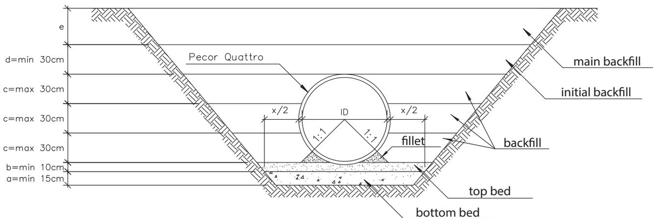
Fig. 6. Applying the bed and backfill for Pecor Quattro pipes
