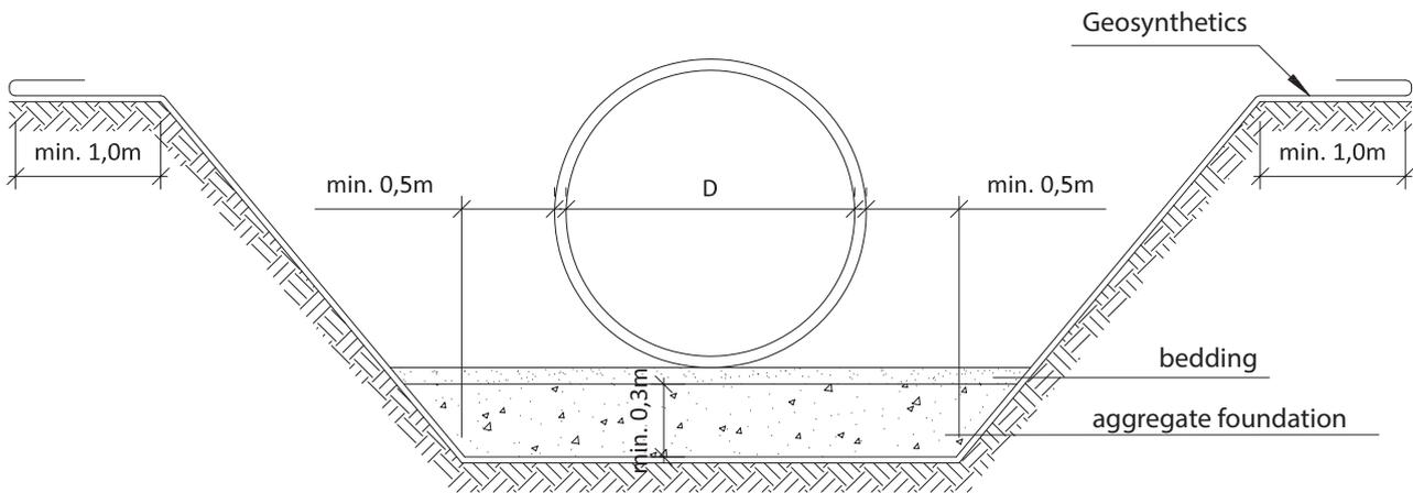
Fig. 7. Laying pipes on low-bearing soil.
