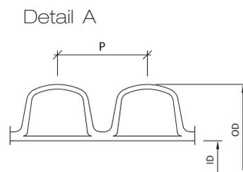
Fig. 2. Pecor Quattro corrugation diagram
