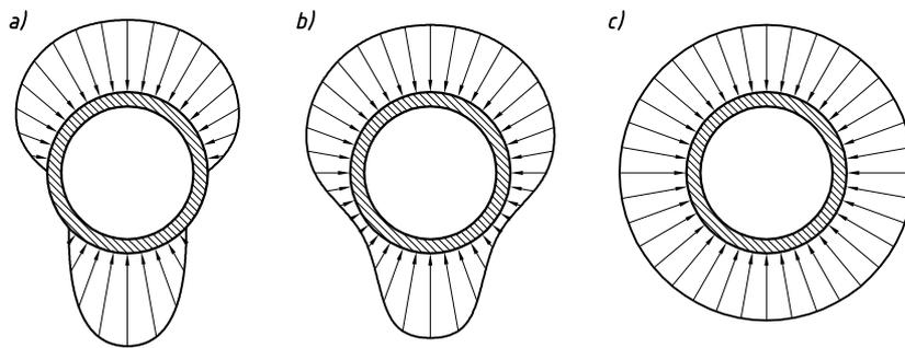
Fig. 9. Load distribution in pipes: a) rigid, b) elastic, c) perfectly flexible, under identical laying and load conditions.
