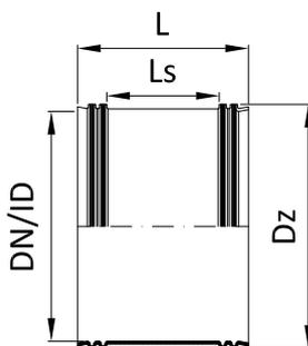
Table 9. Dimensions of Pecor Quattro sleeve connectors
