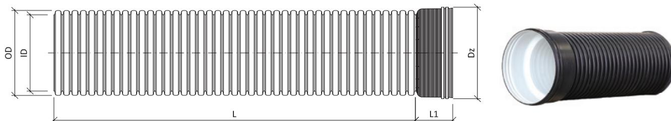
Fig. 3 Pecor Quattro pipes with a socket
