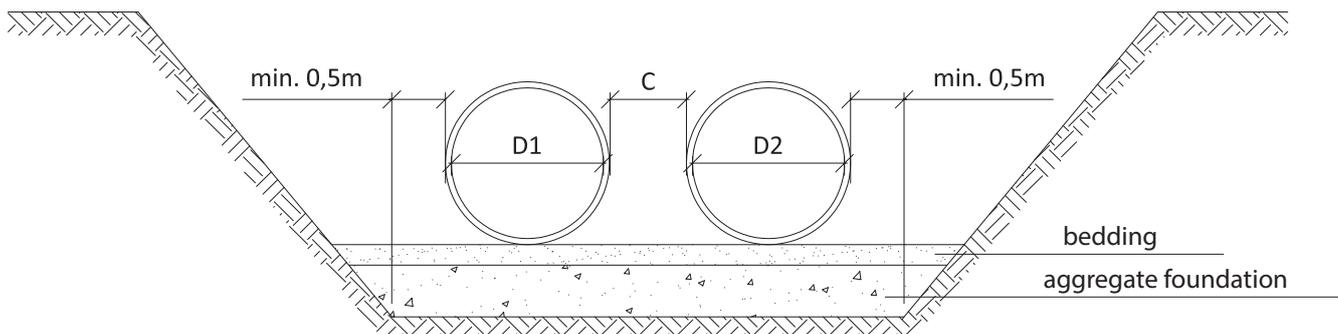
Fig. 8. Distance between pipes laid in the same trench.
